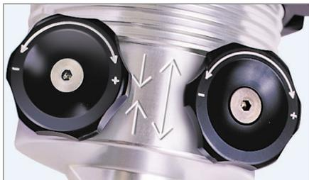
unbolting the VariShock. One knob sets the compression range; the other sets extension. Both knobs are laser-etched with directional arrows and "plus/minus" symbols that clearly indicate which direction achieves the desired adjustment. Additional arrows etched into the QuickSet 2's base reveal which knob sets extension, and which sets compression.
